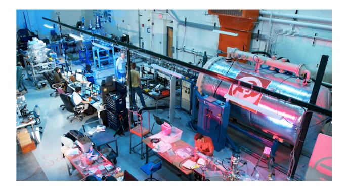
The Institute for Modeling Plasma, Atmospheres, and Cosmic Dust (IMPACT) houses a 3 MV linear electrostatic dust accelerator which is used for a variety of impact research activities as well as calibrating dust instruments for space applications. The dust accelerator is equipped with a 3 MV Pelletron generator capable of accelerating micron and submicron particles of various materials to velocities approaching 100 km/s.
